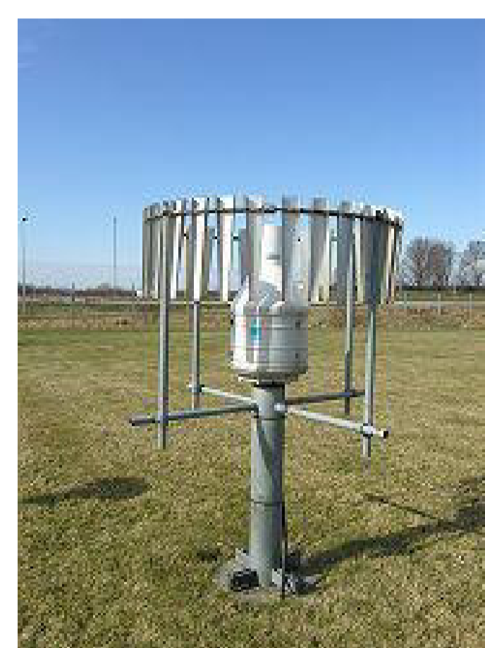
Figure Left: SMHI Gauge with Nipher wind shield. Photo SMHI Right: Geonor Gauge with Alter wind shield. Photo SMHI
