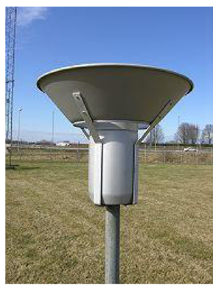
Figure Left: SMHI Gauge with Nipher wind shield. Photo SMHI Right: Geonor Gauge with Alter wind shield. Photo SMHI
