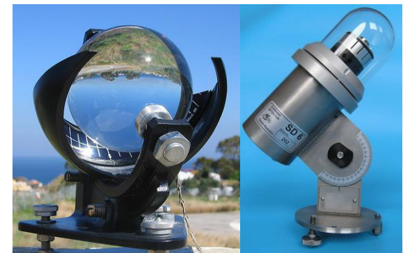
Campbell Stokes heliograph replaced by SDx series of sunshine detectors from Meteoservis Vodňany
