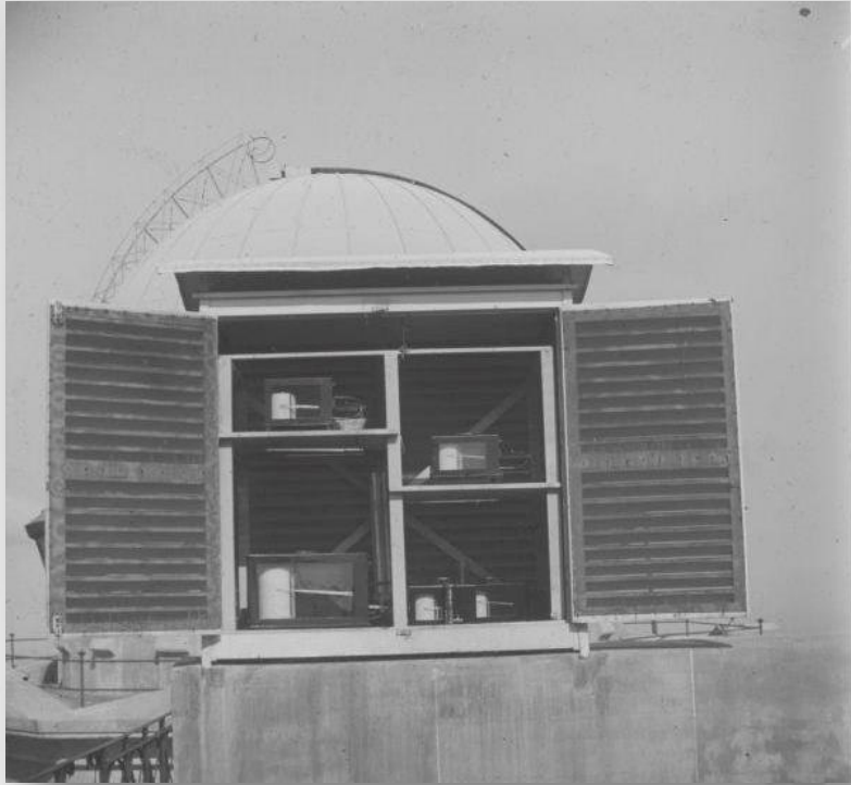
Weekly thermograph and tipping-bucket rain gauge, both Richard manufacturers
