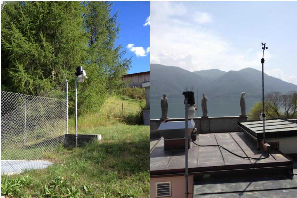
Figure 6: The MeteoGroup stations of Zernez (too close to the forest) and Brissago (station not measuring above grass) are two examples where the stations were relocated to a more representative location due to the results of the METEO-Cert inspections.
