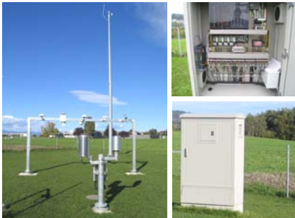
Fig. 1: SwissMetNet – the new automatic meteorological ground-based network of Switzerland
